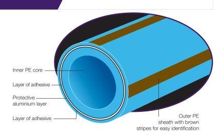
is widely used for the manufacture of potable water pipe systems.
