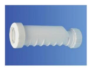
$\mathrm{Hep_VO}^{\$}$  is a self-sealing waste valve for use as an alternative to a traditional water seal trap, in particular where a water seal trap is not suitable, for example, due to climate, movement of the appliance or because of infrequent use. Its in-line design and the option of either horizontal or vertical installation can save space. The valve can also reduce the requirement for additional venting of some appliances.
