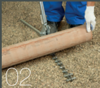
02 Pass the chain under the pipe, aligning the cutting wheels with the desired cut line
