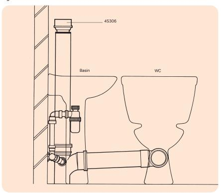
Figure 34: Examples of provisions for drain ventilation
