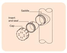
Figure 52: Installation of Access Saddle
