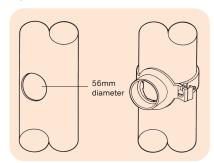
Figure 60: Fitting Boss Socket Adaptor
